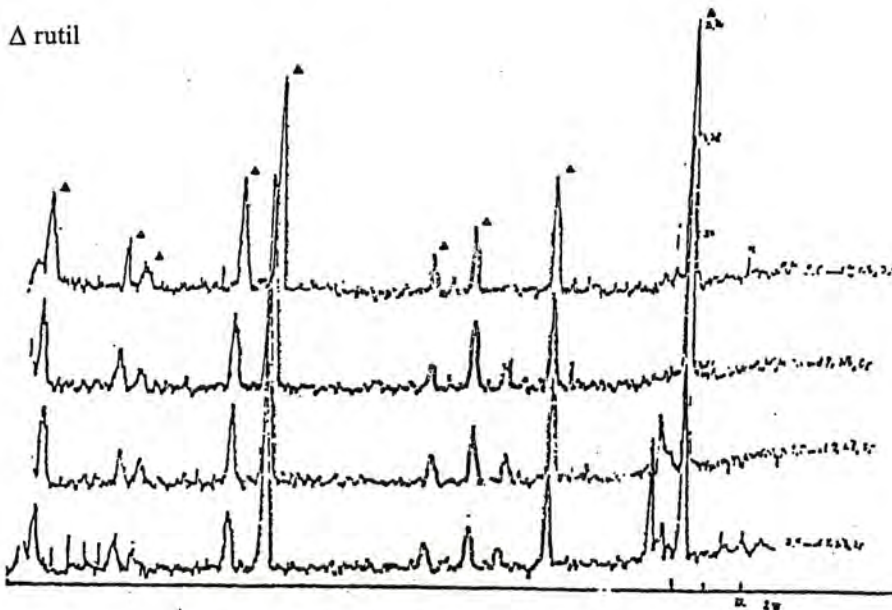
Fig. 2. X-ray analysis of the phases of rutile ceramics of the system \text{TiO}_2 - \text{Nb}_2\text{O}_5
